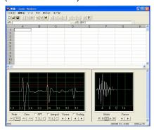
Measure and save waveform (transmission time) of a workpiece of material change to compare the difference from the standard test piece Elastic Modulus Measuring Device is equipped with Pulser/Receiver having the software of Material Surface Sound Diagnosis.
